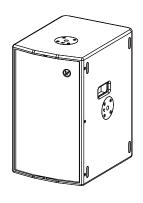
SUB210V series is a high power compact subwoofer made with 2 ferrite magnet 10" drivers that can deliver a peak SPL up to 131dB. The 18mm panels thickness, ports placement and internal bracing stiffens the cabinet structure avoiding undesirable vibrations.
